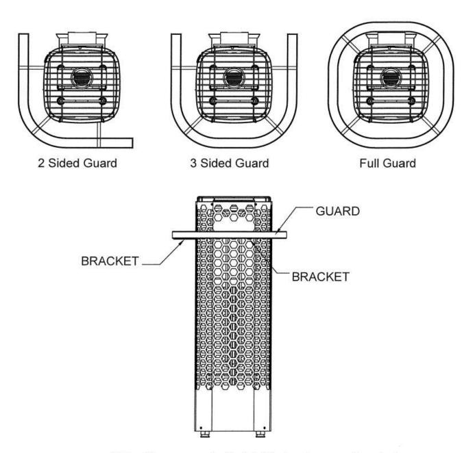
Note: Recommended height for heater guard brackets is 4 holes from top of heater
